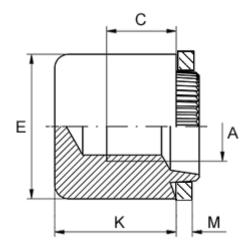
Female thread A = M6Height K = 11.0Min thread length C = 6.0Outer diameter E = 13.0Plate thickness = 2.3 to 2.5
